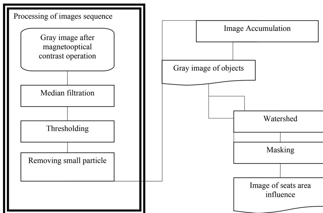
Fig. 5 Pipeline for seat influence area extraction
