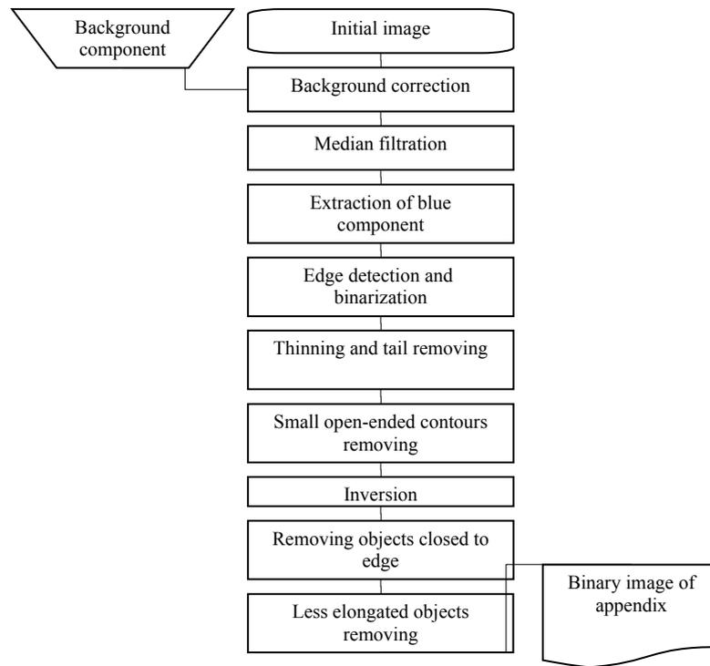
Fig. 3 Algorithm of extraction of appendix on color image
