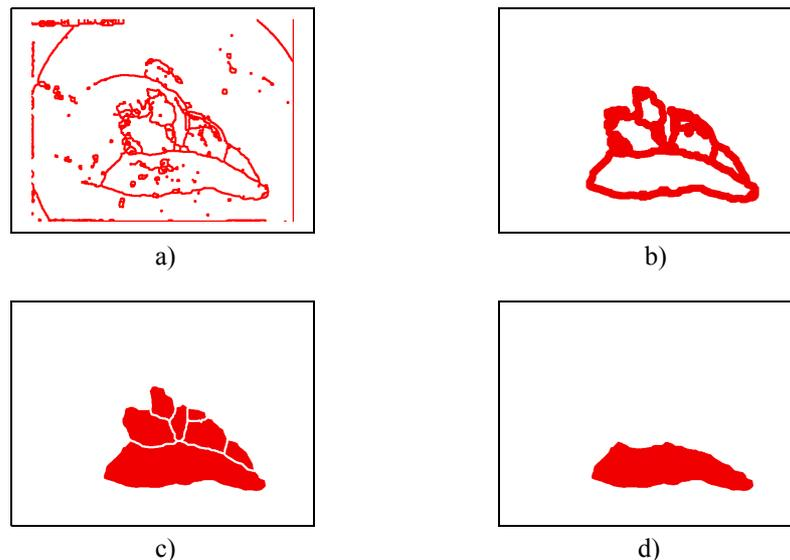
Fig.2 Steps of appendix extraction on binary image: a) borders thinning, b) noise removing, c) extraction of closed regions, d) resulting image of the object
