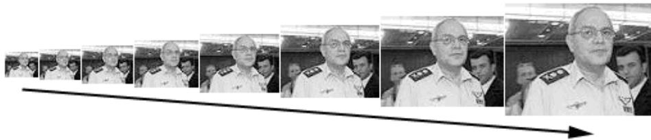
Fig. 3. The image scale pyramid
