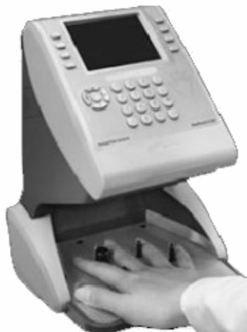
Fig. 1. Palm scanning device
