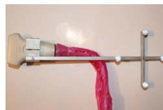
Fig. 2. The US Transducer with four markers
