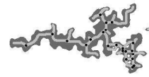
Fig. 5. Topological features of dendrites: gray - dendrites body, light gray - skeleton, black - nodes
