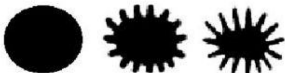
Fig.8 – Objects of different convexity and solidity: convexity and solidity are equal 1; convexity is equal 0,483, solidity - 0,782; convexity is equal 0,349, solidity - 0,592.
